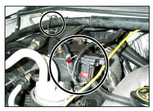
To install the electronic boost cut-off. locate the map sensor located on the passenger side of engine compartment near the rear. Attach the T-Tap or Posi-Tap to the center wire (Light Green/Black trace) and connect the other end to the chassis ground nearby. This device prevents the SES light (high boost code) from appearing.
